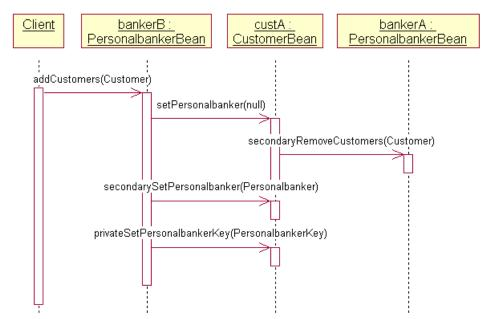
Figure 33. Interaction Diagram for Personalbanker.addCustomers (simplified, only bean implementation specific)
