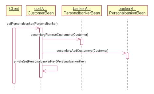
Figure 32. Interaction Diagram for Customer.setPersonalbanker (simplified, only bean implementation specific)
