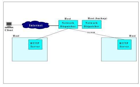
Figure 4. IBM Network Dispatcher
